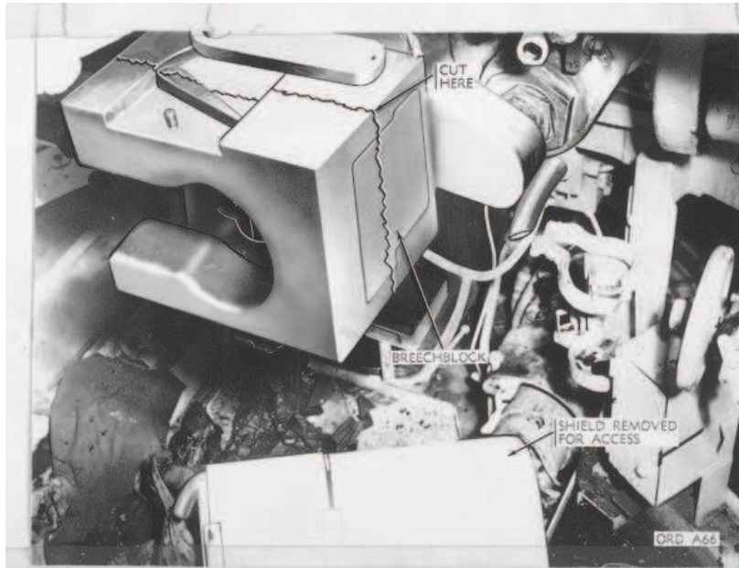
Figure 8. Interrupted Thread Breechblock
